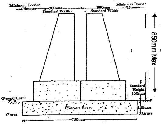
Cross Section of Concrete Beam and Monumental Work Showing
